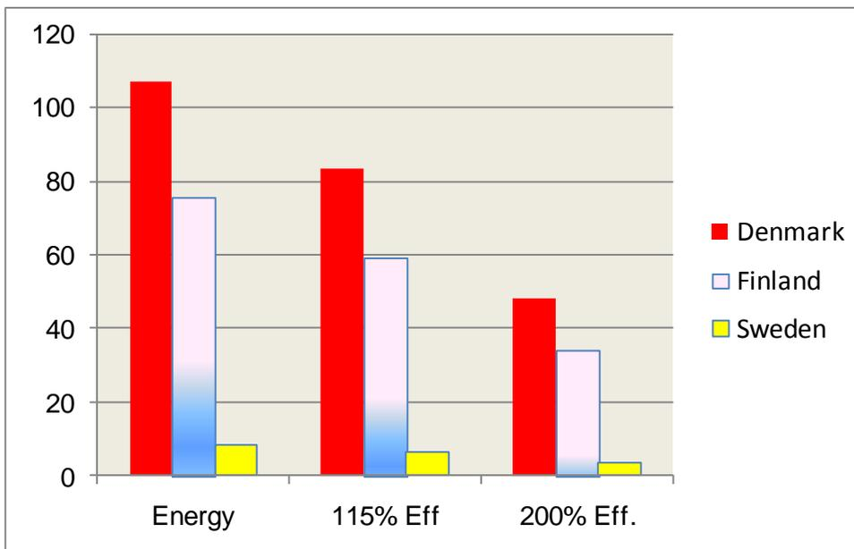
**Figure 8: Comparison of specific CO<sub>2</sub> emission of DH in CHP systems in Denmark, Finland and Sweden with four different allocation methods (g/MJ per CHP heat).**
